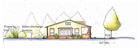
Figure 4.3-B: Illustration of Drainage on Lot
