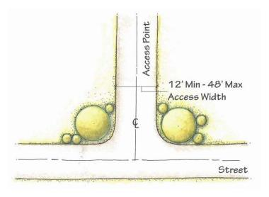
Figure 5.3-F: Illustration of the access width measurement
