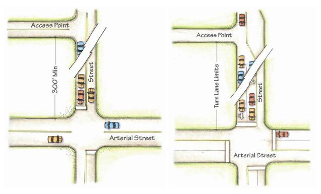
Figure 5.3-B: Illustration of access spacing from Arterial Streets
