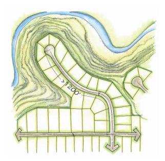
Figure 4.1-T: Illustration of where Cul-de-sacs may be appropriate due to topographic conditions
