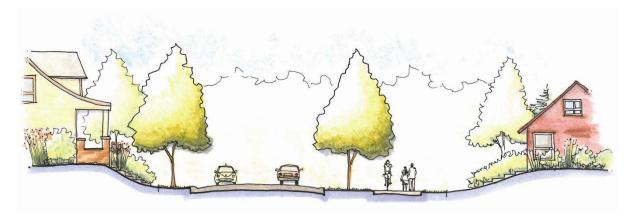
Figure 4.1-D: Typical cross-section of a suburban development arterial street without parking
