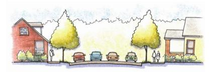
Figure 4.1-I: Typical cross-section of an urban development subcollector street with parking on both sides of the street
