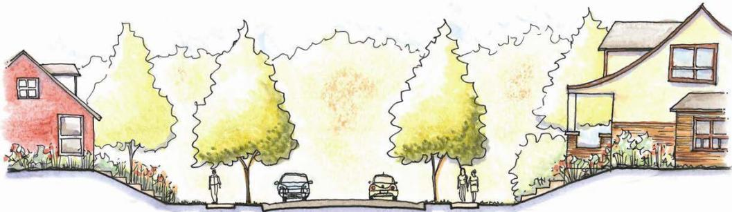
*Figure 4.1-C: Typical cross-section of a suburban development collector street without parking*
