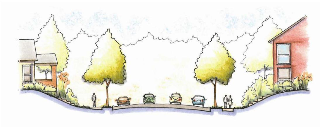
*Figure 4.1-G: Typical cross-section of a suburban development subcollector street with parking on both sides of the street*
