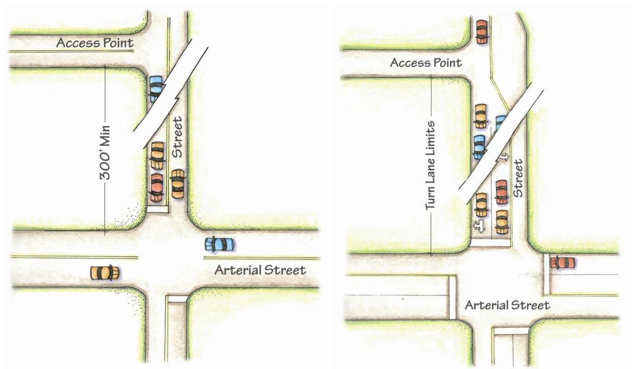
Figure 5.3-B: Illustration of access spacing from Arterial Streets
